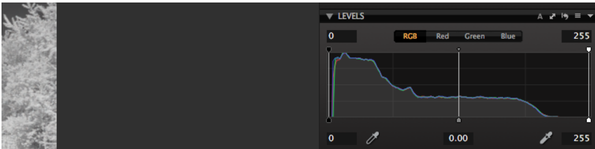
IR picture histogram. Note how all the color channels are on top of one another.
