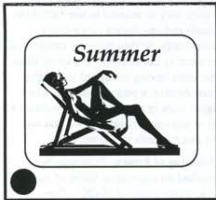
FRONT of slide as viewed normally, with thumb spot in lower left corner
